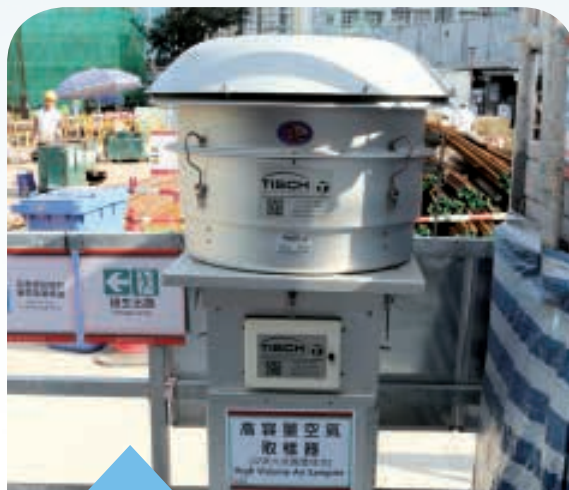
High volume air sample collector to track the air quality at construction sites
